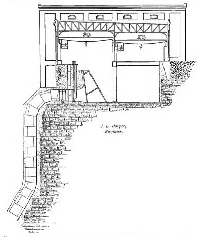
FIG. 126. Section of the head house of the power plant of the Niagara Falls Hyd. Power and Mfg. Co.
